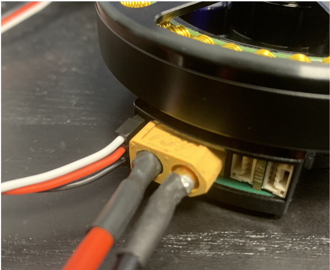
Motor with power and UART connections
